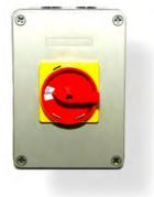
Available in 32 and 63 Amp ratings Rear mounted in IP65 grey ABS plastic enclosure. Padlocking device (max. 3 padlocks) prevents the switch from being turned ON by unauthorized personnel Interlock provided so lid can only be opened in OFF position Red/yellow handle colour
